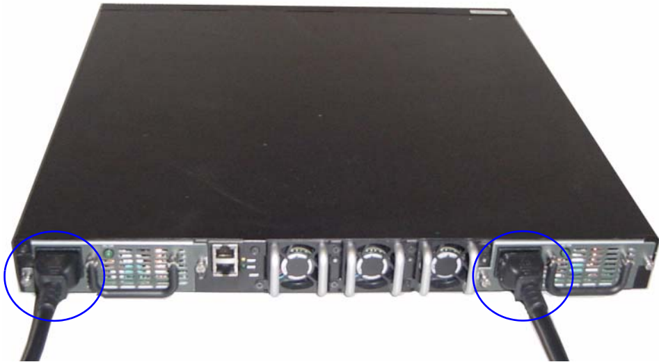
Figure 2. Connecting Power Cables
